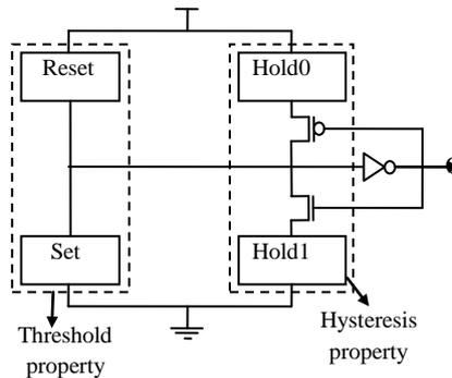
Figure 4: Static NCL gate topology
