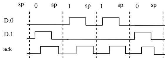
Figure 3: RTZ 1-of-2 data transmission.
